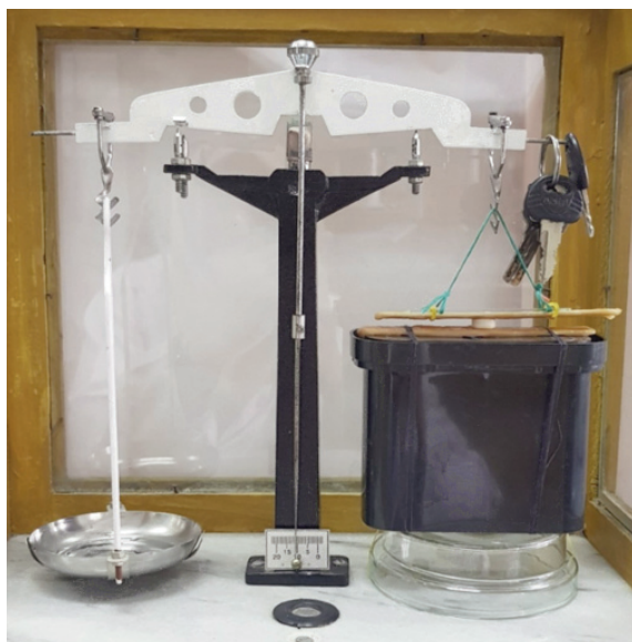
Figure 1. Depiction of the reconstructed mucoadhesive strength tester for the measurement of mucoadhesive strength as reported 30 in the literature.
