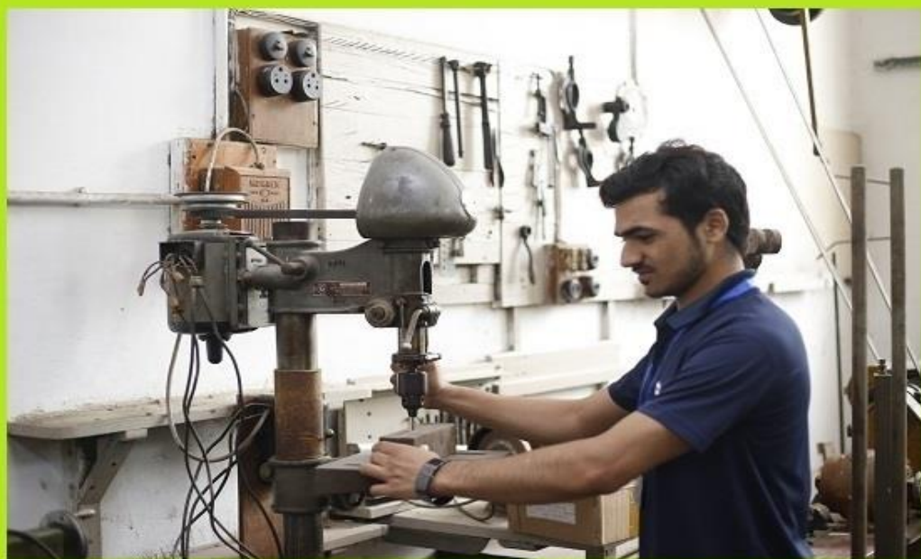
Mr. Danish employing the Drilling-Threading Machine to repair apparatus
