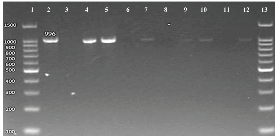
FIGURE 3: Molecular detection of ESBLs ( bla CTX-M-15 ) gene (996 bp). Number 1 and 13: 100 bp DNA ladder; number 2: positive control; number 3, 6, 8, 11: negative samples; number 4, 5, 7, 9, 10, 12: positive samples.
