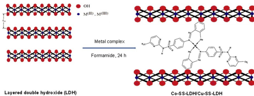
Figure 5. Formation of metal complexes with layered double hydroxides via intercalation. Reprinted with permission from reference [8] Copyright 2019, open access, Elsevier.
